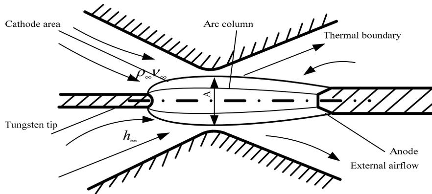
Figure 2: Schematic diagram of arc discharging model.
