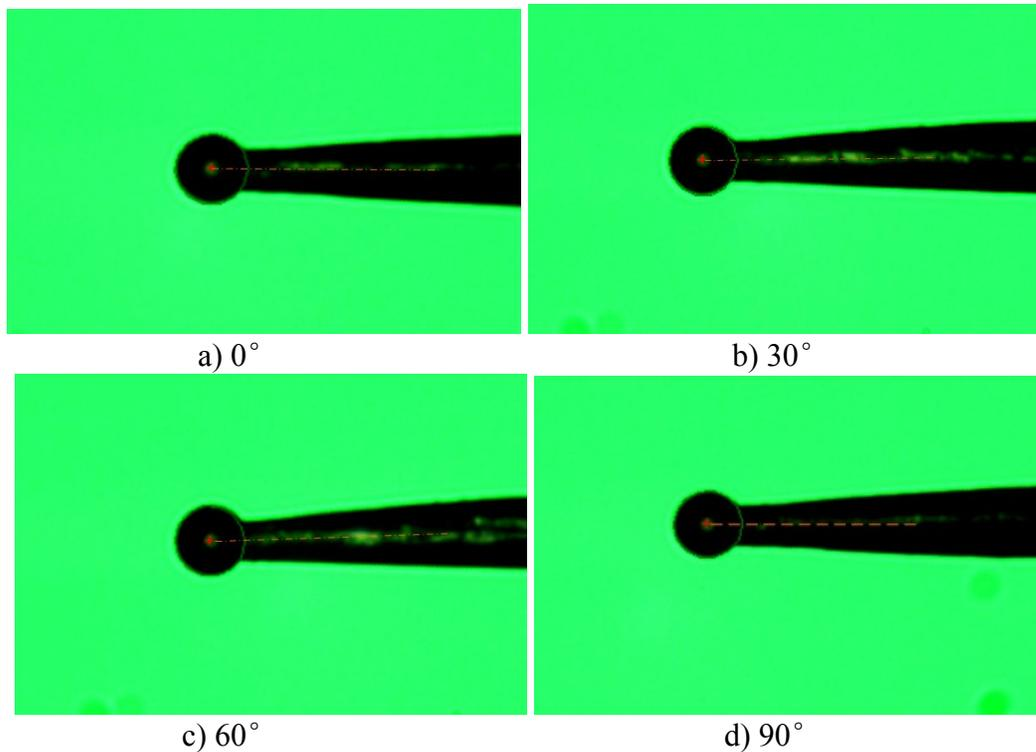
Figure 6: Images of a tungsten tip viewed from different aspect angle.
