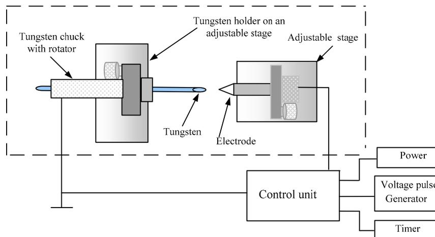
Figure 3: Experimental configuration for fabricating tungsten probe.
