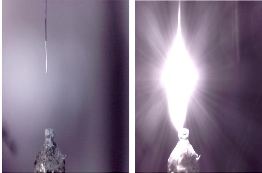
Figure 4: Image of fabrication of tungsten tip, (left) before sparkling, (right) in process.
